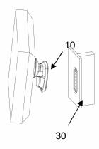
Figure 12. Attach Mount to Wall Bracket
